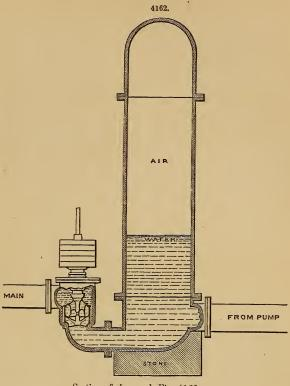
Section of air-vessel, Fig. 4161.
